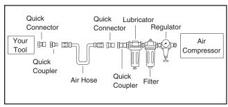
Figure 2. Installing your tool.
